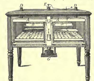
Incubator. A, hot-air tank; B, tray for holding pans of water; C, C, egg-trays; D, D, ventilators; E, automatic regulator; F, rod connecting thermostat with regulator; G, lamp; H, thermostat; I, thermometer.
